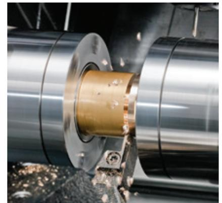
Spindle No. 2 is on the B-Axis and is servo motor driven for thrust and feedrate to help provide high precision movement and easy set-up. This feature alone can save up to 20% in operating efficiency over conventional designs.
