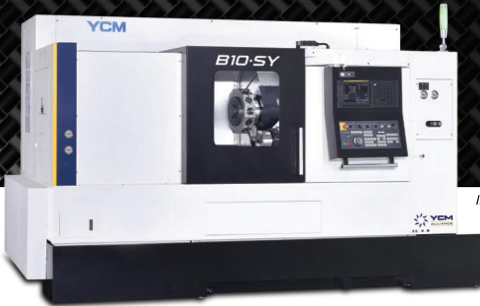
Mid-high range 6-axes machine (X/Y/Z/B/C1/C2-axes, live tooling and sub spindle) for middle to upper range components.
