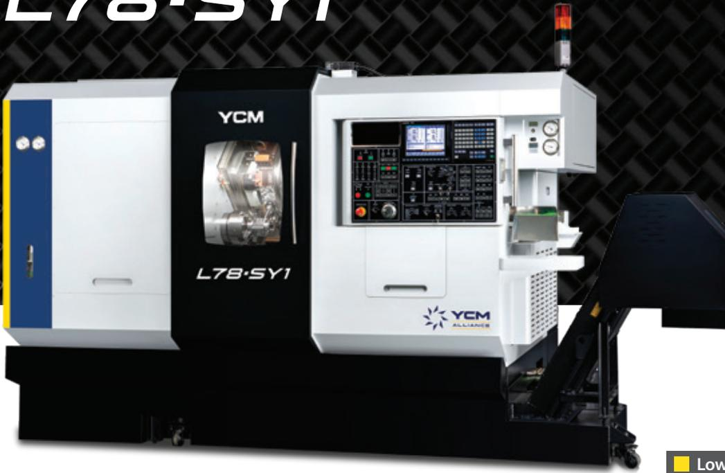
Mid-high range 8-axes machine (X1/X2/Y/Z1/Z2/B/C1/C2-axes, 2 x 16 stations, live tooling and twin spindles) for middle to high range components.
