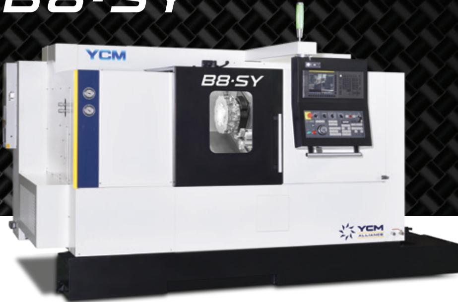
Mid-high range 6-axes machine (X/Y/Z/B/C1/C2 C2-axes, live tooling and sub spindle) for middle to upper range components.
