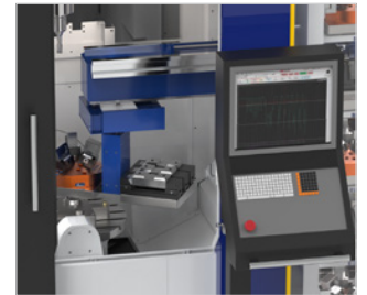
Quick pallet exchange – load arm holds two pallets for quick exchange of the completed pallet and the new pallet.
